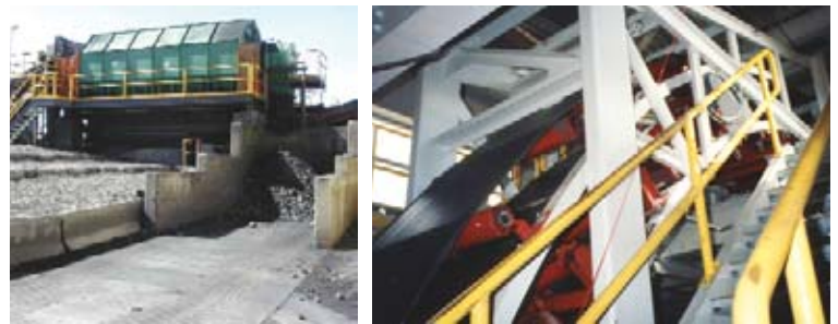
Nucla uses a rotary breaker (left) to prepare coal and a high-angle conveyor (right) to carry it to a rooftop extension of the stoker boiler building.
