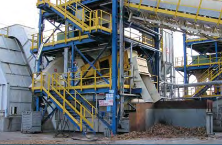
▲ ENEL burns biomass with coal at a plant on Sardinia. Shown are the yard bin and biomass handling and processing systems.
