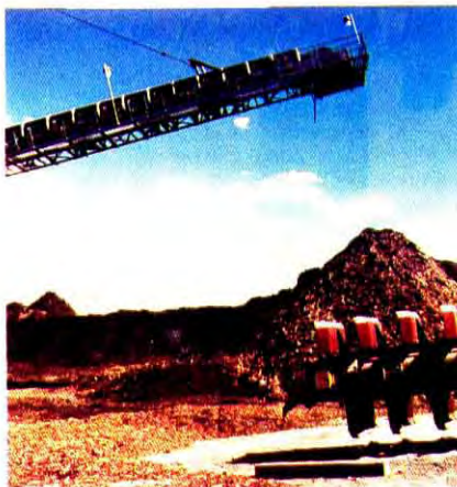
5. Wood chips are reclaimed from kidney-shaped pile by underpile drag-chain reclaimer or boom-type overpile drag-chain reclaimer
