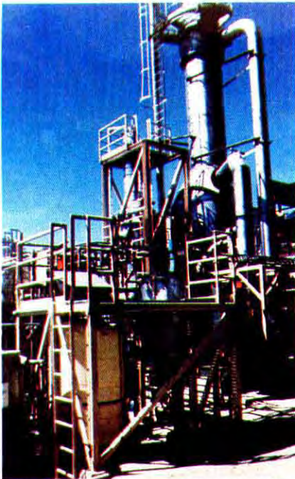
3. Water treatment system features brine concentrator and leased demineralizers
